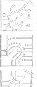
The images to the left illustrate three conceptual subdivision layouts. The top image is an example of a poor layout with too few connections and many dead ends. The lower two images show improved street layouts with the required connections and a network of streets. (Diagrams courtesy of Fort Collins Colorado)
