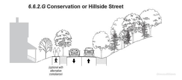
Definition: Streets designed to accommodate environmental constraints and to encourage minimal grading and adaption to the natural character of the land. This street standard can be applied when environmental issues, environmental protection and/ or conservation are a consideration. This standard can only be used with the preapproval of the administrator.
