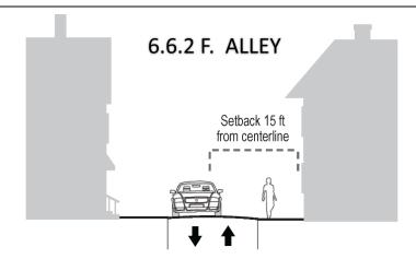
Definition: Alleys are intended to provide indirect, limited access to the rear of properties but not to accommodate through traffic. Utilities, either above ground or underground, may be located in alleyways to provide service connections to rear elevations.
